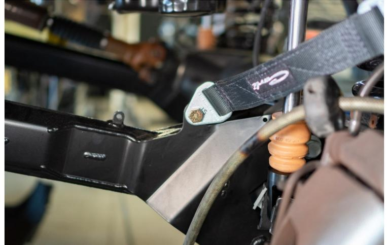
6. Pull the strap up against the frame rail ensuring the strap is parallel to the shock and fully stretched. Make a mark in the center of the hole with the strap pulled tight.
