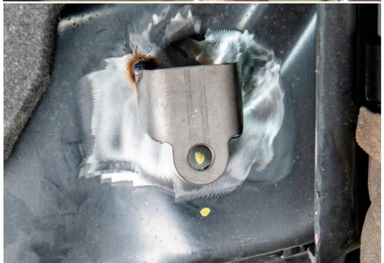
13. Once confirmed, fully weld both sides of the tab.
