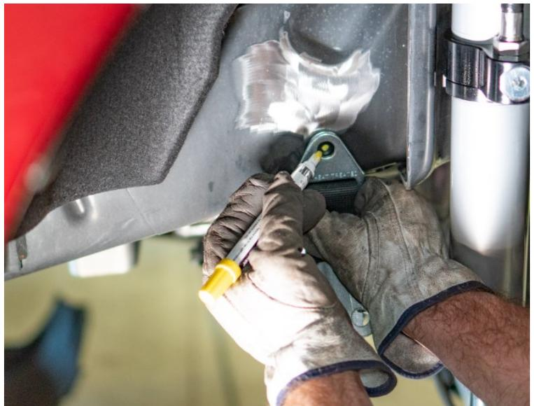
9. Measure 1" up from the mark you just made on the frame (in line with the path of the limit strap) and make a new mark. *This accounts for the break-in and stretch of the limit strap.*
