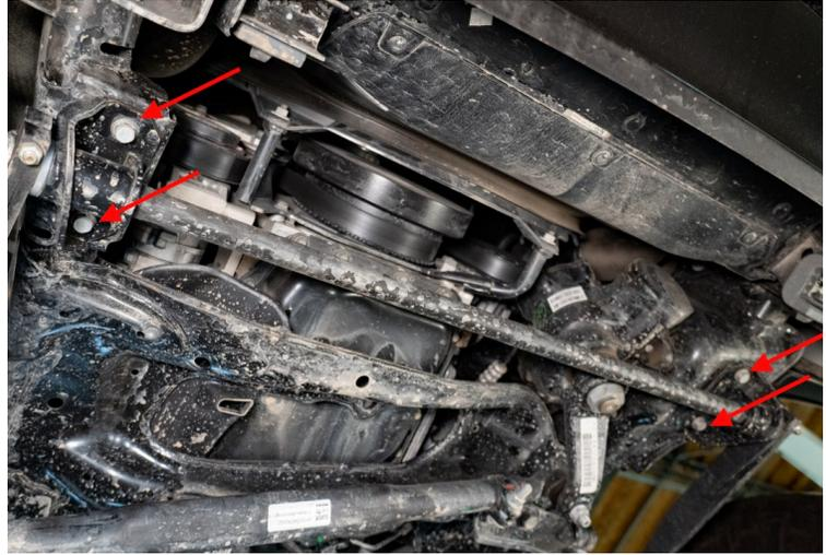
2. Insert the provided sway bar spacer between the sway bar bracket and frame rail.
