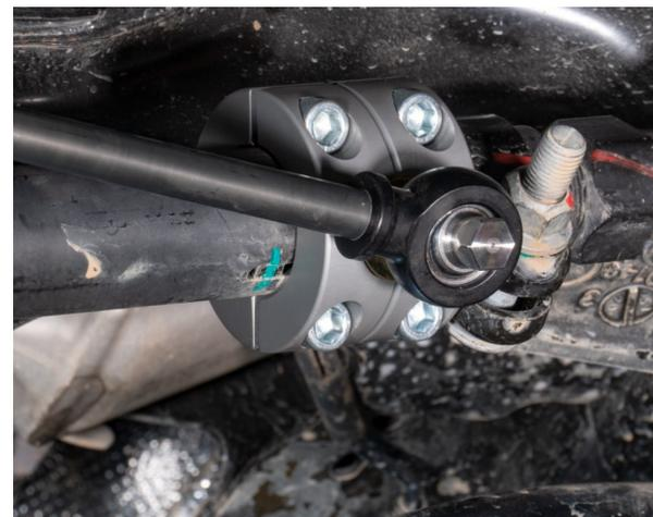
13. **CLAMP ORIENTATION:** At this point, the installation is complete aside from the hand-tight allen heads on the clamp and final stud torquing. Set the truck on the ground if the installation was performed in the air, and straighten the wheels.
