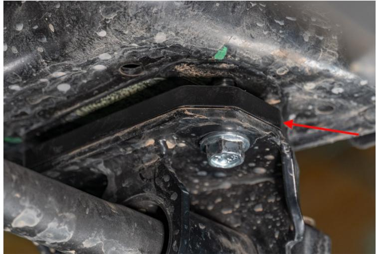
4. Install the Passenger side stabilizer shock mount between the sway bar bracket and frame rail securing with the remaining M10 x 40mm bolts.
