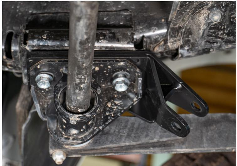
7. Index the clamp to the adjustment collar of the drag link.
